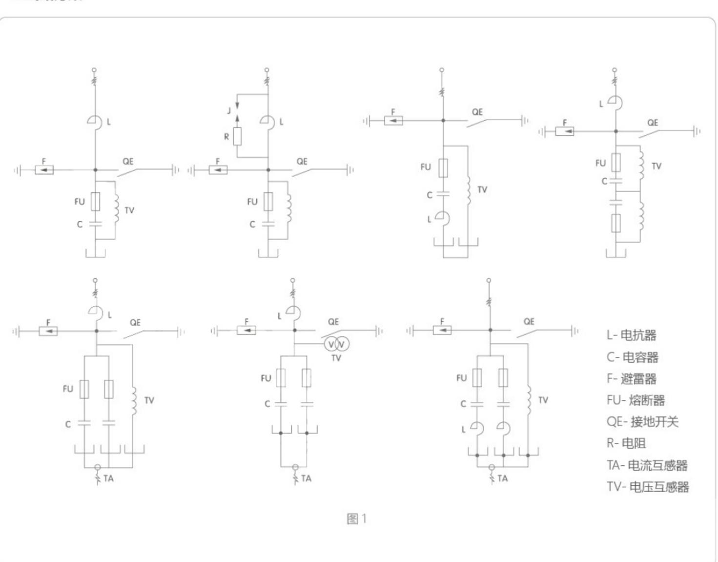
The typical primary circuit scheme of this device is shown in Figure 1, where the grounding switch is installed according to user requirements. When
